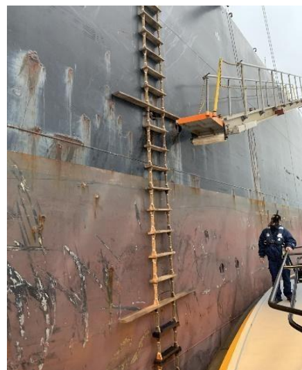
Inboard stanchion missing, ladder & gangway not secured to hull.
